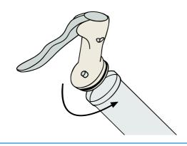
3) Attach the cone to the opposite, open end of the cylinder.
