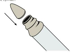
4) Start with the pubic ring diameter 20, and slide it onto the open end of the cylinder using the cone and a little lubricant. Remove the cone. If this ring is too large, try out the next smaller ring.
