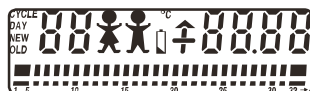
Fig. no. 7 The unit performs a function test after start-up, all the display elements are shown.
